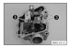
Install and tighten the screws
