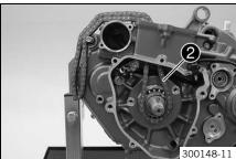
Thread the timing chain ② in and lay it over the timing chain sprocket.
