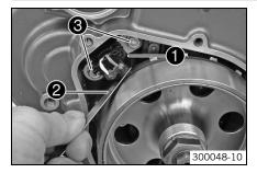
Adjust the distance between the crankshaft position sensor • and the conductive element of the rotor using the special tool •.
