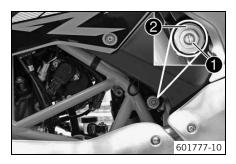
Turn adjusting screw • clockwise with a screwdriver up to the last perceptible click.
