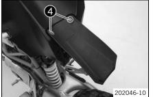
Position the splash protector. Mount and tighten screws 4.
