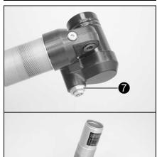
Remove compression adjuster •. Remove the spring, sleeve, and piston.
