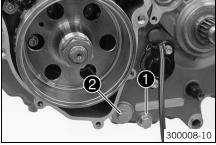
Mount the oil drain plug • with the magnet and a new seal ring and tighten it.
