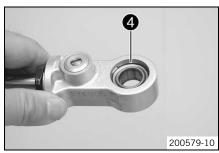
Remove lock rings 4 on both sides.
