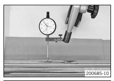
Measure the run-out of the inner tube.
