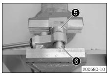
Place special tool **⑤** underneath and press out the heim joint with special tool **⑥**.
