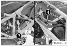
Plug in connector 3 of the lambda sensor. Position the cable and secure it with cable binder 4.
