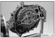
Clamp the antihopping clutch with special tool ①.
