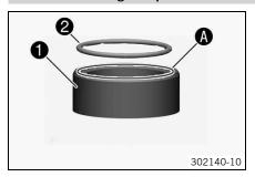
Grease spacer • in area • and O-ring • before mounting.
