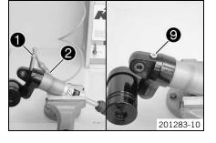
When the pressure gauge reaches the specified value, turn the Damper control lever 4 to Pressure.
