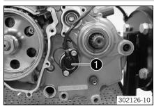
Remove screws. Remove the gear position sensor •.
