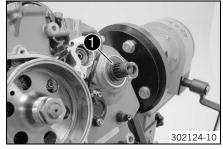
Grease the shaft seal ring.
