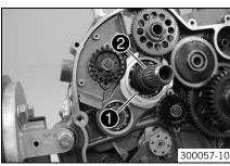
Install supporting plate 1 and needle bearing 2.
