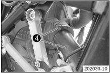
Remove nuts 4 of the manifold.
