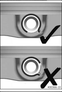
Position the piston pin retainer.
