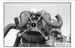
Put the valve cover in place with the seal. Mount and tighten screws ①.
