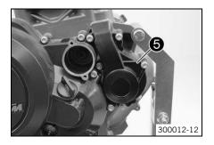
Put on the water pump cover **3**. Mount and tighten screws.
