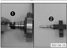
Mount the special tool **1** on the alternator side of the crankshaft.
