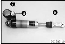
Grease O-ring of the seal ring retainer.
