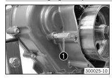
Set the crankshaft to top dead center and lock it with the special tool ①.
