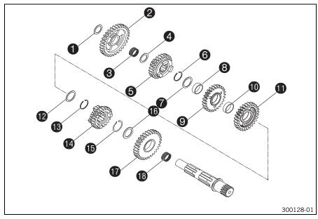
Fix the countershaft in the vise with the geared end facing downward.
