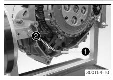
Install the spacer 1 and spring 2 of the shift shaft.
