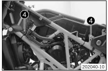
Mount and tighten screws 4.
