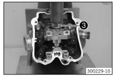
Press in the large camshaft bearing as far as possible using the special tool 4.
