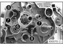
Mount the oil pump gears ⑤, washers ⑥ and lock washers ⑥.
