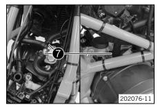
Position the hoses of the engine breather, the SLS and the oil return line. Mount the spring band clamp vising the special tool.
