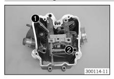
Position the rocker arm 1 and push in the rocker arm shafts 2.
