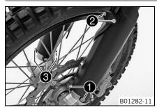
Position the fork protector on the left fork leg. Mount and tighten screws ①.
