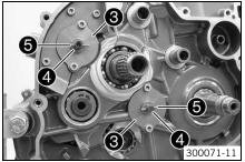
Position both oil pump covers **3**. Mount and tighten the screws.
