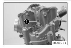
Mount and tighten the spark plug • using the special tool.
