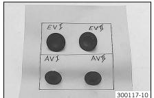
Mark the valves according to their normal built-in position.
