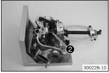
Press in the small camshaft bearing as far as possible using the special tool 3.
