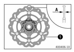
Check the thickness of the front and rear brake discs in several places to ensure that it conforms to measurement .
