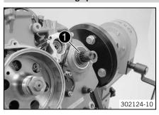
Remove the spacer • of the countershaft.
