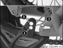
Remove screws 1 and 2. Take off the chain guide.
