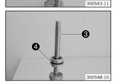
Position special tool 3 on the piston rod.
