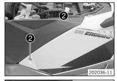
Mount and tighten screws ②.
