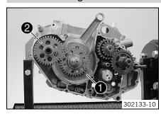
Remove the crankshaft 1 and the balancer shaft 2.
