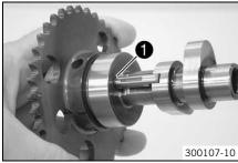
Take the lock ring ● off the autodecompression shaft and dispose of it.
