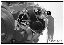
Remove screws 1. Take off the water pump cover.
