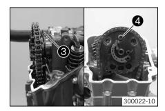
Position the camshaft support plate 3. Mount and tighten screw 4.
