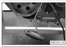
Push the oil screen with O-rings on to a pin wrench. Push the pin wrench through the opening into the drill hole of the opposite engine case wall and push the oil screen as far as possible into the engine case.
