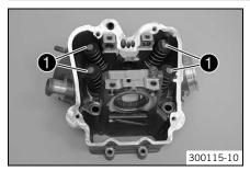
Take shims • out of the valve spring retainers and lay them to one side according to their normal built-in position.
