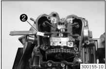
Check the valve clearance on all valves between the valve and the rocker arm using the special tool ②.
