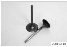
Check the run-out at the valve plate.
