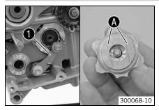
Press locking lever • down and position shift drum locating.
