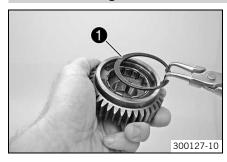
Extract the lock ring • from the groove using suitable pliers.
