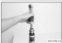
Remove the piston rod. Drain the remaining oil.
