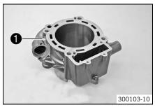
The cylinder size • is marked on the side of the cylinder.
