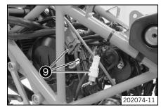
Plug in connector 9 of the gear position sensor, the crankshaft position sensor, and the alternator.
