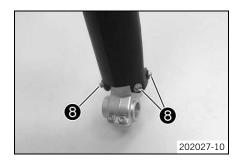
Remove screws 3. Remove the fork protector from above.
