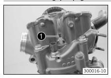
Remove the spark plug using the special tool •.
