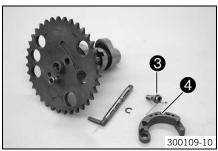
Disconnect the autodecompression spring. Loosen the screw ③ and remove it together with the autodecompression spring and the autodecompression weight ④.
