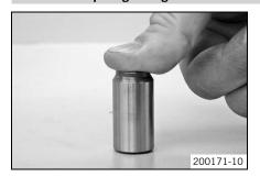
Fully compress the timing chain tensioner.
