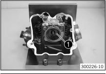
Remove the small camshaft bearing using special tool 2.
