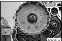
Install the clutch cage 3.
