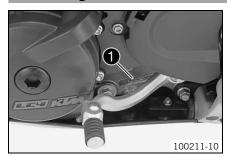
The engine number  $m{0}$  is stamped on the left side of the engine under the engine sprocket.
