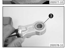
Remove seal rings 3 on both sides.
