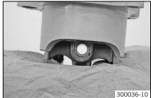
Cover the engine case opening with a cloth. Thread the timing chain through the chain shaft. Mount the piston pin.
