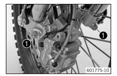
Turn adjusting screws 1 clockwise all the way.
