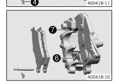
Check that leaf spring 3 in the brake caliper and sliding plate 7 in the brake caliper support are seated correctly.
