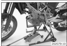
Position the floor jack under the engine and fix it using the special tool.
