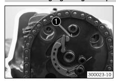
Turn the crankshaft counterclockwise until markings ● of the camshafts are flush with the marks of the camshaft support plate.
