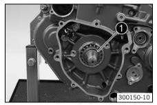
Heat the timing chain sprocket and push it immediately on to the crankshaft.
