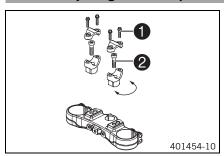
Remove the four screws ①. Remove the handlebar clamp. Remove the handlebar and lay it to one side.
