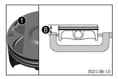
Measure the piston at the piston skirt, at right angles to the piston pin, at a distance <sup>3</sup>
