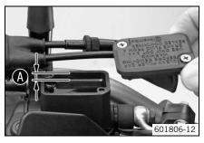
Adjust the brake fluid level to level **a**.
