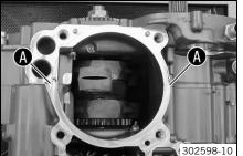
Apply a thin layer of sealing compound in area ...
