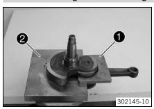
Fix the crankshaft with special tools 1 and 2 in the vise.
