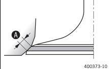
Check sealing seat **(A)** of the valves.
