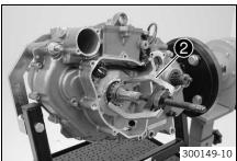
Pull of the timing chain sprocket with the special tool 2.
