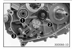
Push sliding plate 1 away from the shift drum locating 2. Remove shift shaft 3 with the washer.
